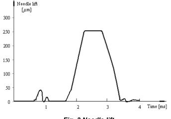
Fig. 3 Needle lift
