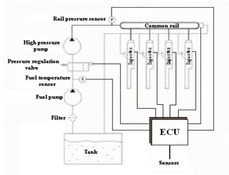
Fig.1 Common rail injection system
