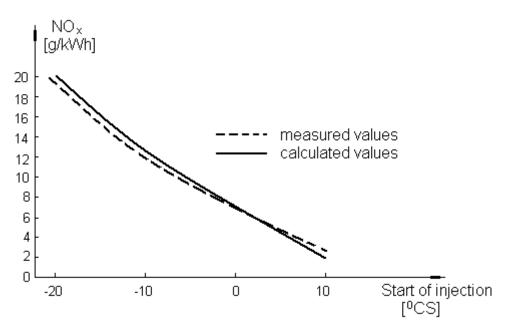
Fig.4 Comparison between measured and calculated values for nitrogen oxides
